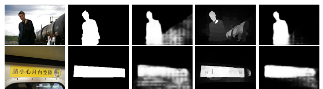
Fig. 3: Benefit of integrating deep and unsupervised saliency. From left to right: Input image, ground truth, results of deep model, RBD and our deep-shallow integrated model.
